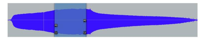
As you can see in the above waveform, the loop is placed where the volume is at a fairly even peak and the EQ spectrum is at its brightest as well.
