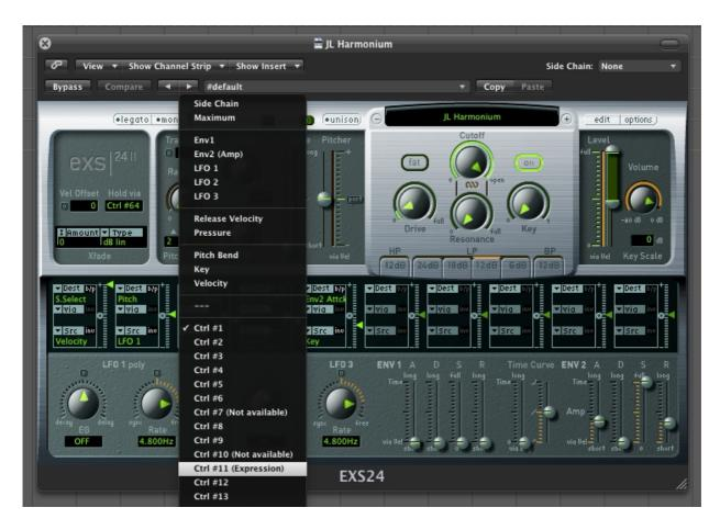
Simply click on the green Ctrl#1 in the matrix for the Rel. Volume and a drop down menu will appear. As you can see above – just select Ctrl #11 (Expression Pedal) as the Src (source). The do the same thing for the Filter Cutoff as well. Be sure to save the instrument afterwards. Of course you can choose any controller in the list as well.
